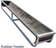
50NB M Gal pipe. 650mm (w) x 500mm (h) x 4000mm (l). Rust free rubber trough self draining.
